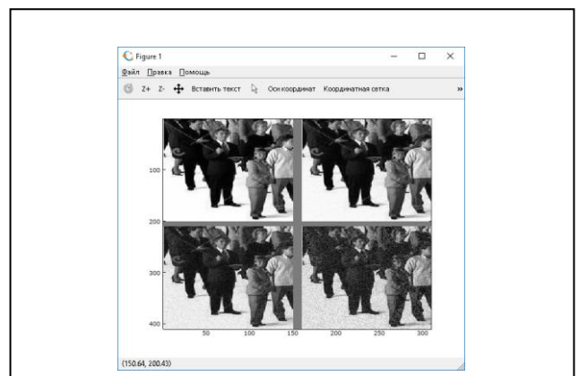
Fig. 3. An example of distortions in the image of a live queue, there is noise
