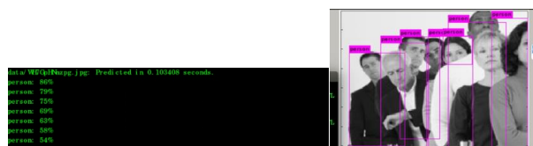
Fig. 9. Result of image processing in YOLOv3
