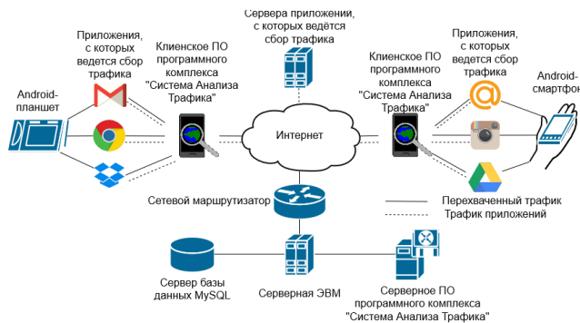
Fig. 1. Scheme of collecting mobile traffic
